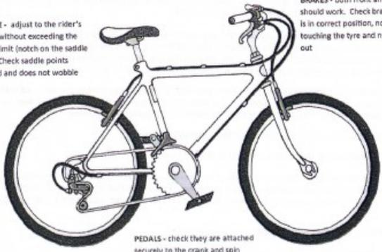
**SADDLE** - adjust to the rider's height without exceeding the safety limit (notch on the saddle post). Check saddle points forward and does not wobble
